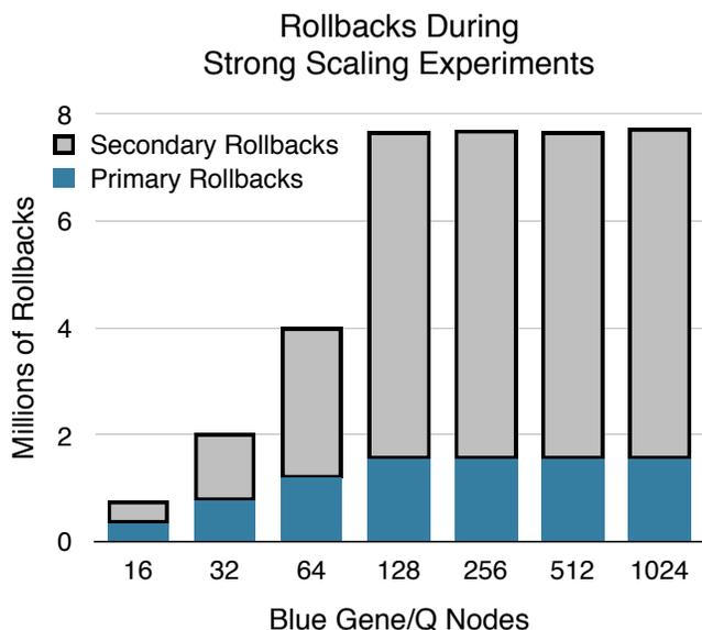
Figure 11: Breakdown of the primary and secondary rollbacks for the strong scaling simulation. Note that the net event population for these experiments is 13 billion events, but the maximum number of rollbacks observed is only 7.6 million.
