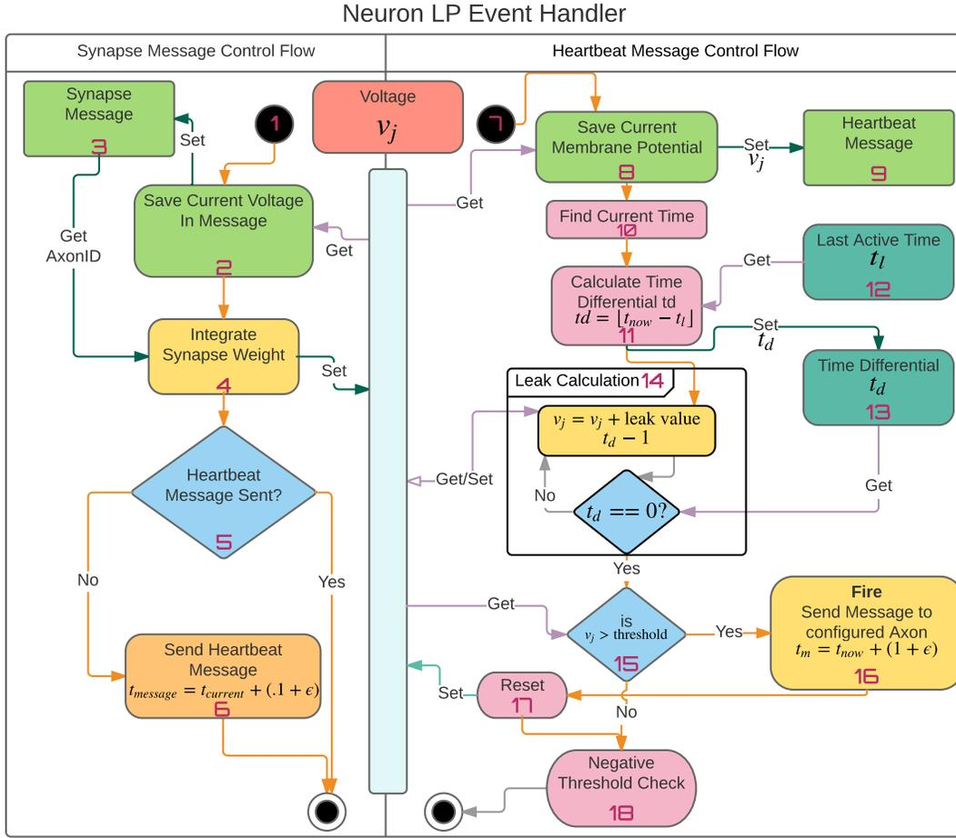
**Figure 3: The *NeMo* neuron event flow.** Details of each block, numbered 1 through 18, are discussed in Section 3.1.
