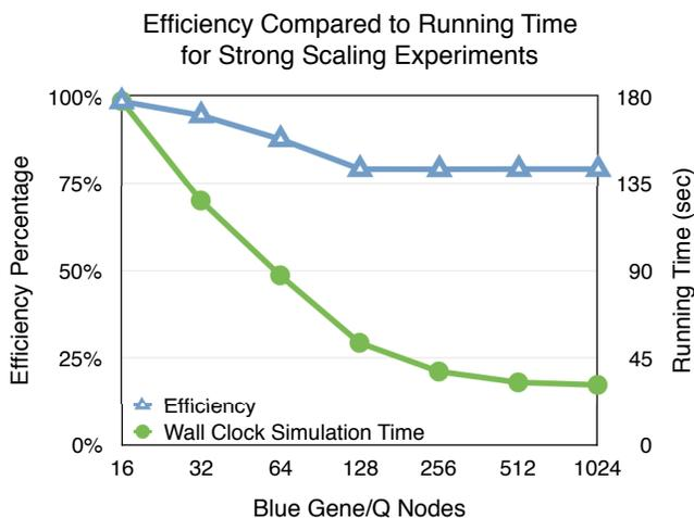
Figure 10: Comparison of the efficiency and the running time of the strong scaling experiments.
